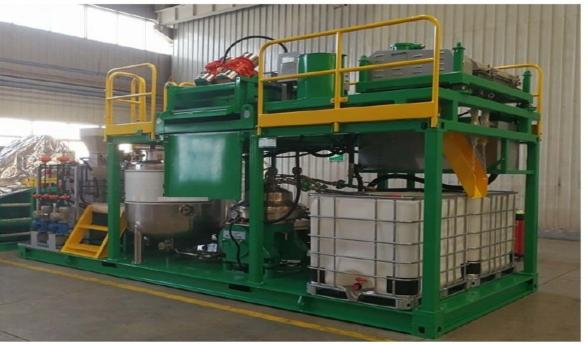
The above unit is a test unit with capacity of 2m³/h, Dimension: 8000\*2786\*3257 mm
